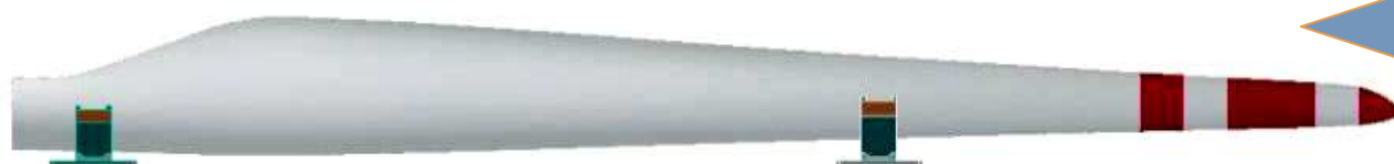
Typical 2.4MW 44.7m Blade Weight : 8 ton All GFRP
