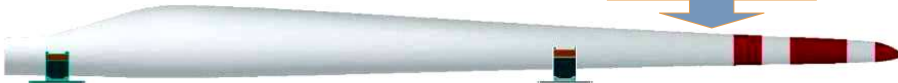
Typical 5MW 56.5m Blade Weight : 32 ton GFRP + CF Spar Cap
